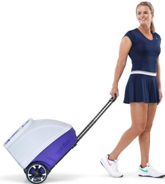
To transport in your car, please make sure the machine is always kept upright. Laying it on its side can cause internal damage and void your warranty. Do not store the machine in your car when external temperatures exceed 30 degrees Celsius (86 degrees Fahrenheit). The machine weighs 24 kg (53lbs) (or 18 kg (40lbs) with an external battery) and should be lifted carefully with the use of the handles.
